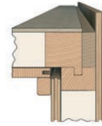
3. Wall to ceiling connection with deep-groove joint.
